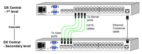
Figure 30 Example of cascaded DX Central units
